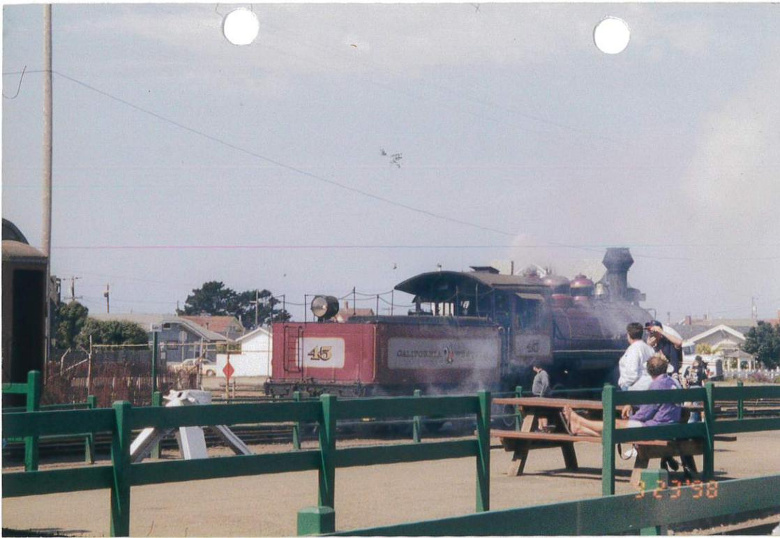
1. Locomotive #45 (steam engine) currently burning used/recycled oil as a fuel.
