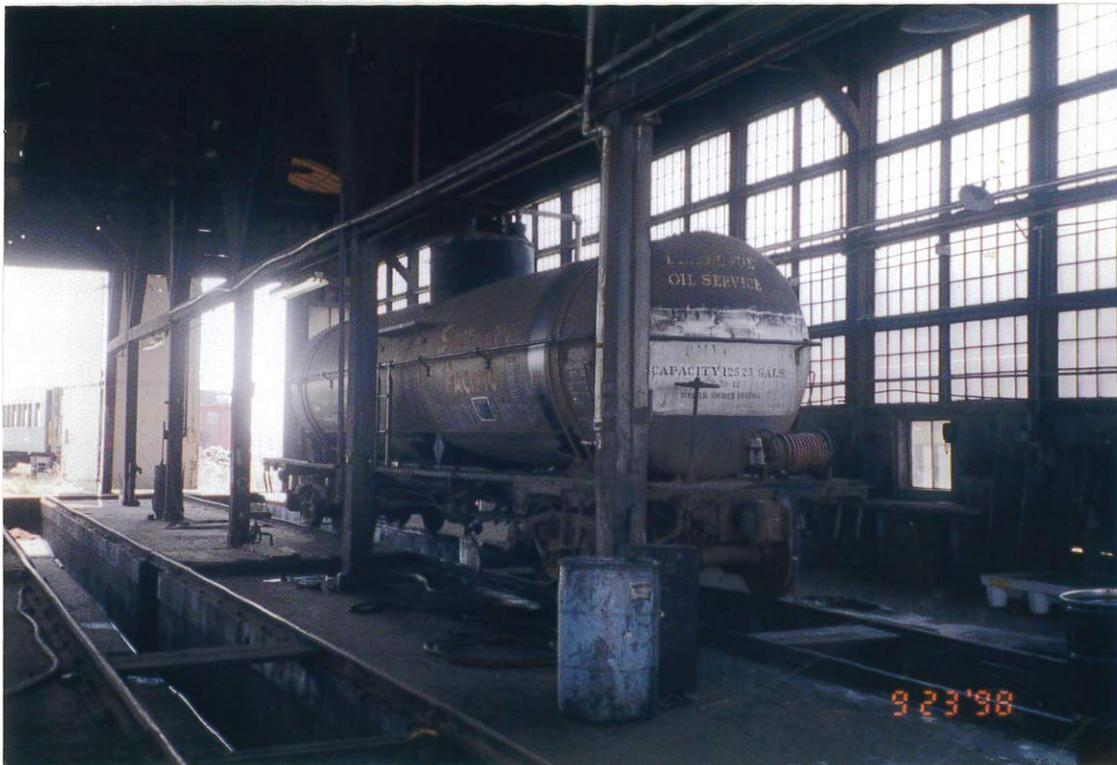
2. Railcar inside of the "roundhouse" used to store used/recycled oil. Lower right-hand corner of photo shows open unlabeled drum of oily sludge cleaned from the trench.
